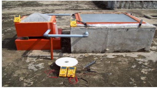
Fig (3) Pyramid Solar Still with Shallow Solar Pond with insulation
