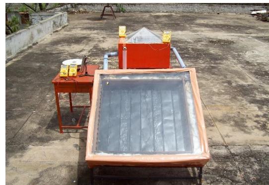
Fig (2) Pyramid Solar Still with Flat Plate Collector with insulation
